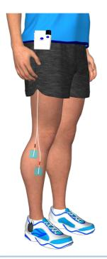
The ODFS® Pace XL uses a wireless connection between the footswitch and the stimulator. This removes the need for a footswitch wire running down the leg.
