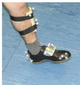
*Figure 1: Kinematic marker arrangement*
